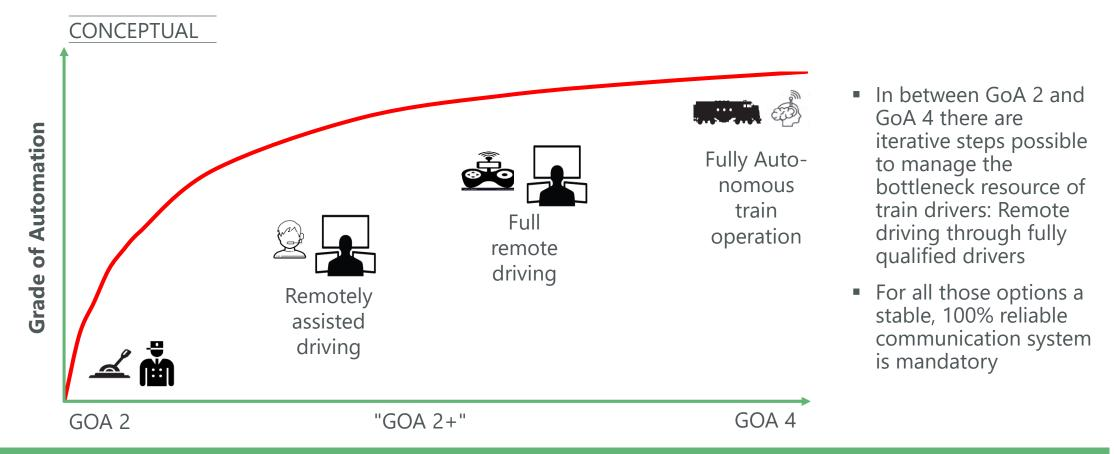
Iterative and cycle-wise ATO migration steps are necessary to speed up the automation process, benefit from short "lessons learnt"-cycles and deliver quick solution for freight with the best quality and performance ("low hanging fruits")
