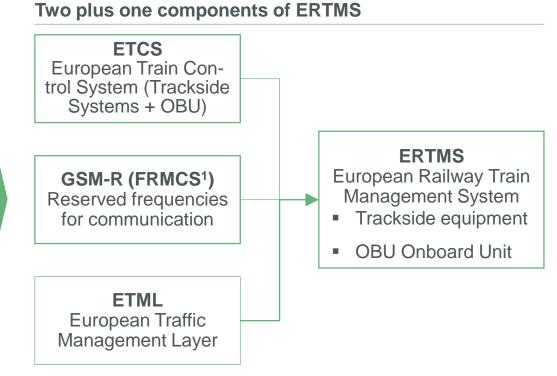
**Technically enabled SERA**<sup>2</sup> ("Single European Rail Area") by implementing **one standard ERTMS** both on trackside as well as OBU (Onboard units) including established and working processes (ETML)
