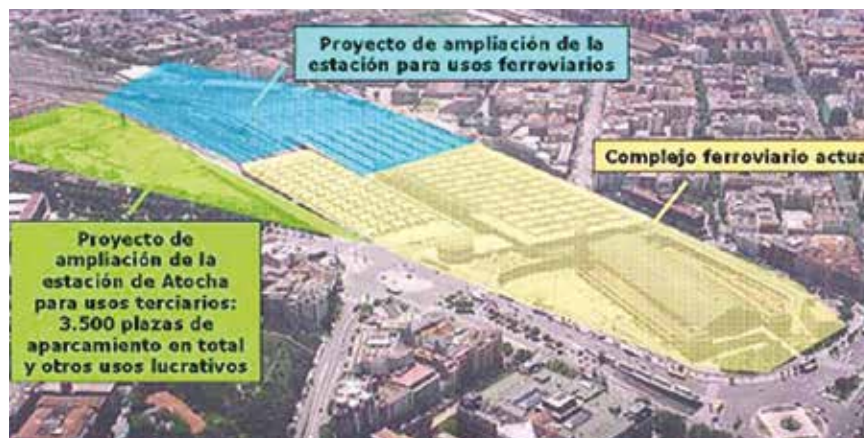
Site coverage of station extension in 2010. From left to right: Project to expand Atocha Railway Station for tertiary purposes: a total of 3,500 parking spaces and other commercial purposes (in green); Project to expand the station for rail purposes (in blue); Existing railway complex (in yellow). Source : Adif.
