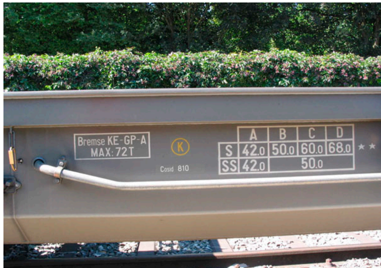
Figure 3.1. Freight wagons equipped with K-blocks with indication on the side of the car.
