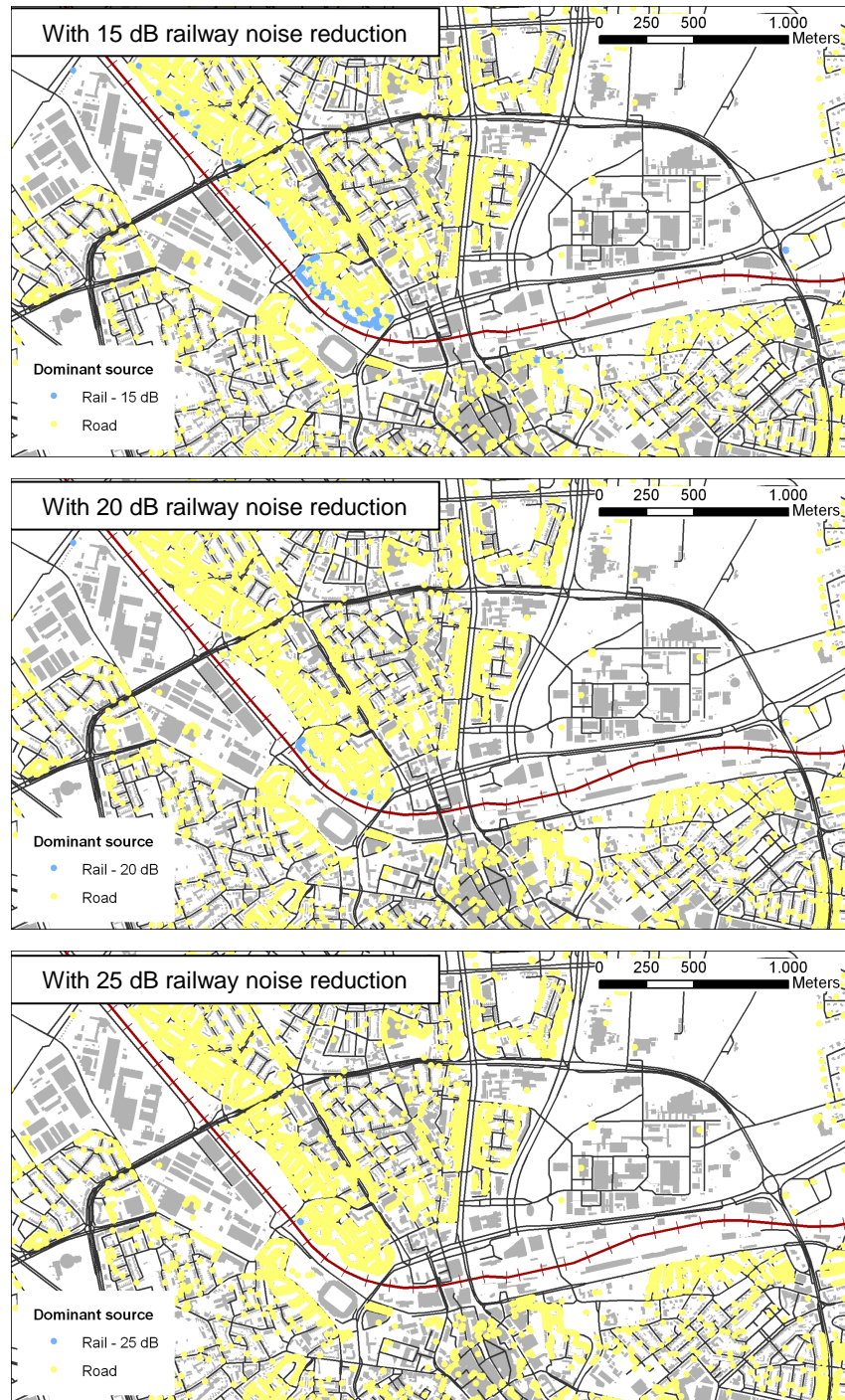
Figure 23b Dominant source for the number of sleep disturbed persons for situations with 15, 20 and 25 dB noise reduction.
