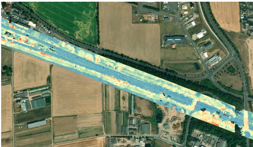
Figure 35: Mapping lineside tree populations using satellite data and artificial intelligence to identify potentially hazardous trees near the line, © Deutsche Bahn AG / LiveEO
