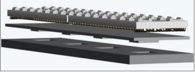
Targeting the drainage probl em between lines in subgra de section, the horizontal dr ainage channel is set betwe en the bases, which reduce bad influence of drainage fa cilities on subgrade and dur ability of track structure.
