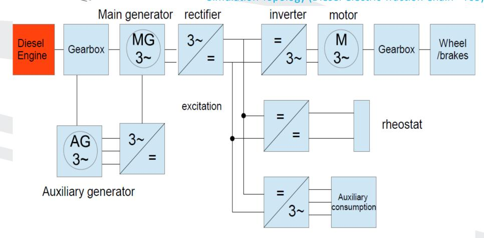
**Diesel electric traction**
