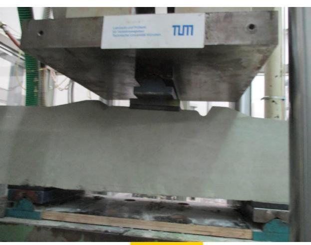
Fig. Test setup for the examination with positive bending moment at the rail seat
