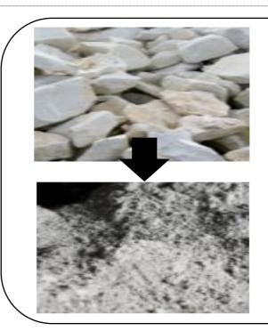
To produce cement, limestone needs to be heated up to 1,450 °C in order to separate  $CO_2$  from lime.
