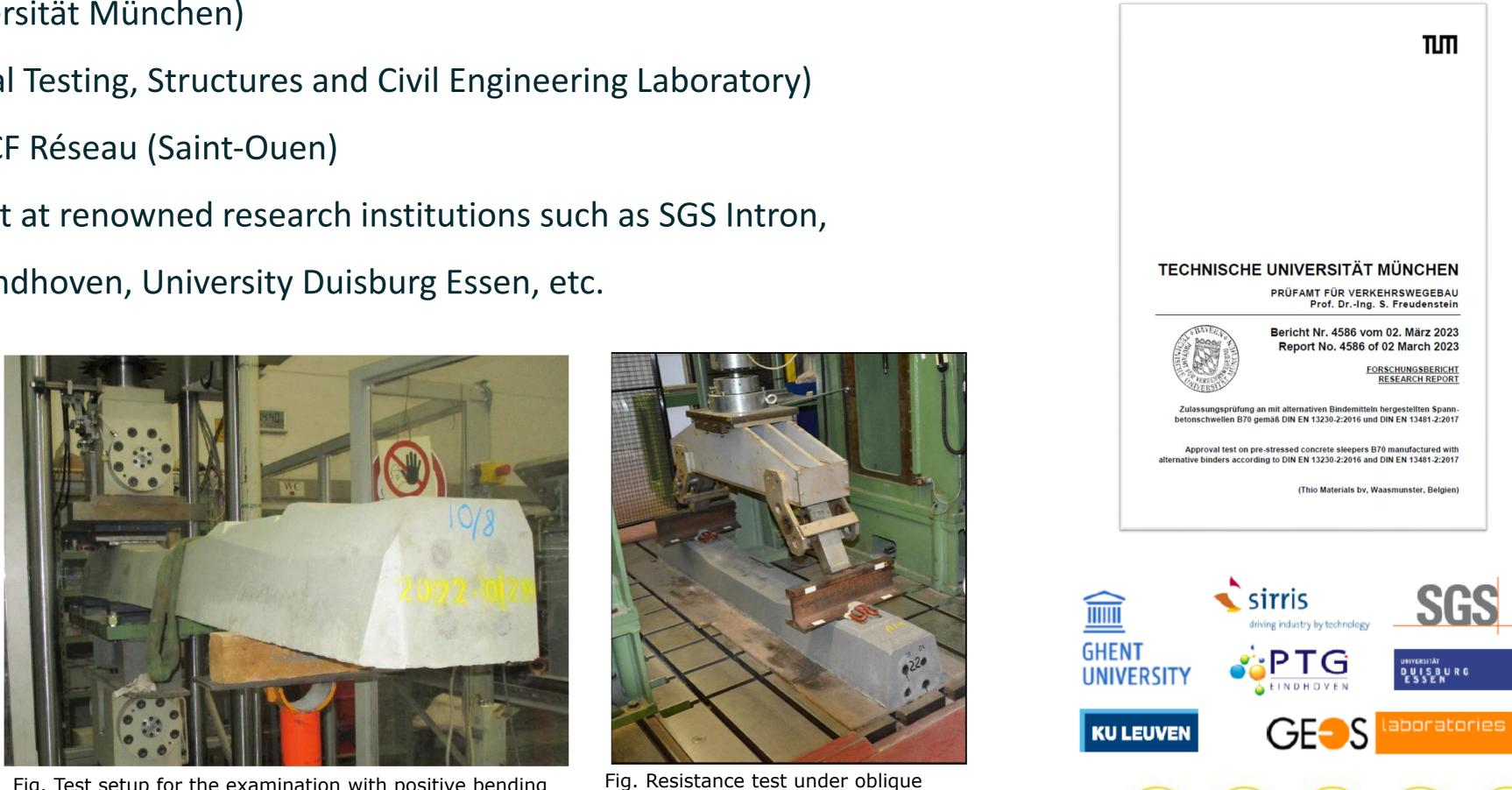
Fig. Test setup for the examination with positive bending moment at the rail support
