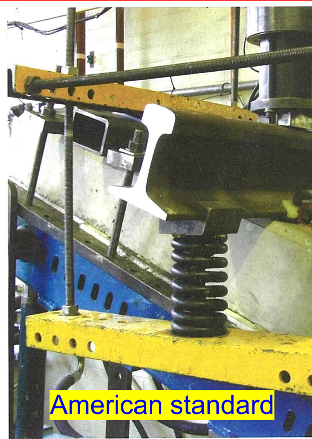
Testing of fastening systems according to European (left), American (centre) and Japanese (right) standards.
