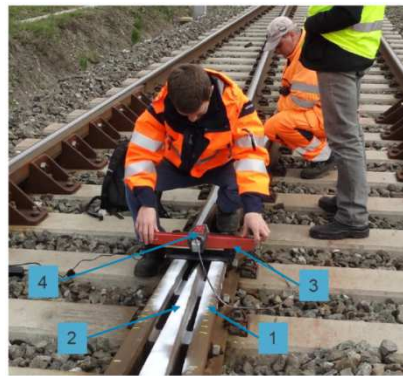
Figure 12: Switch panel measurements and alignment
