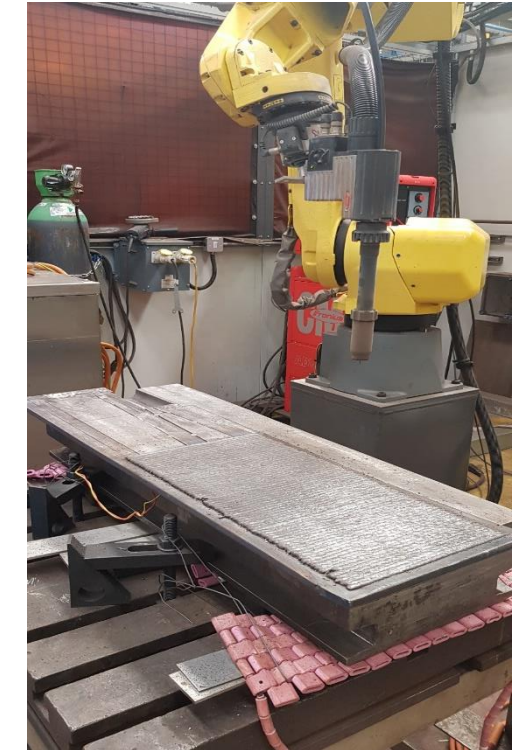
Photograph showing the weld deposition process
