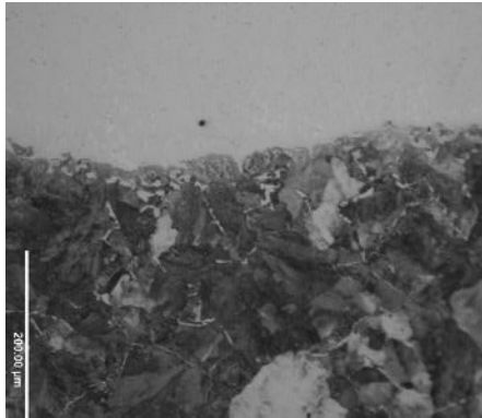
Clad (top, white) to substrate (bottom, grain structure) fully bonded interface
