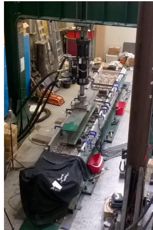
2. A testing apparatus has been modified for long bearer testing
