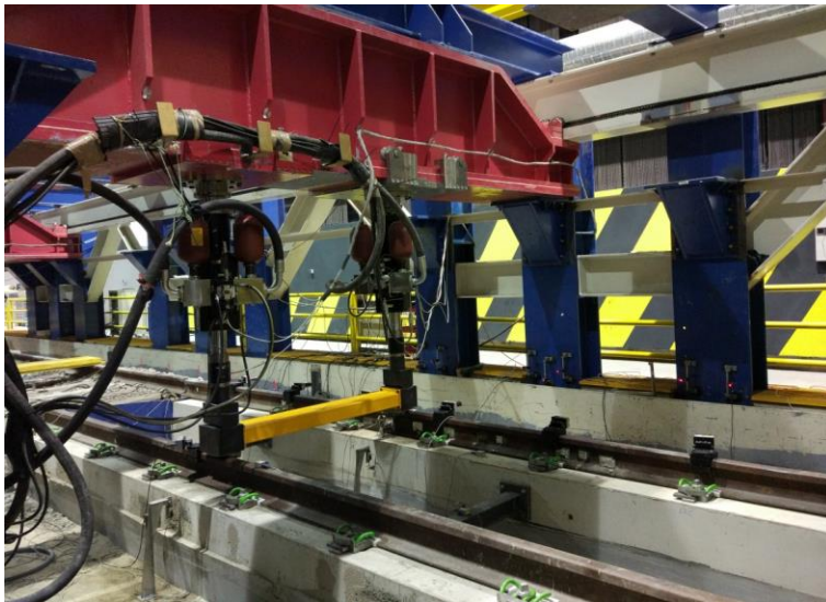
Hydraulic actuators during the static test
