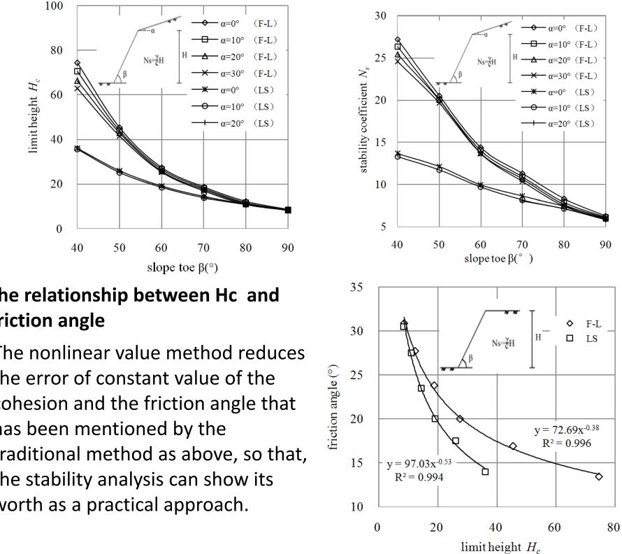
(1) the gradient of curve decreases with the increase of stress, and (2) the friction angle becomes smaller as it is concerned with the nature of undisturbed loess itself.
