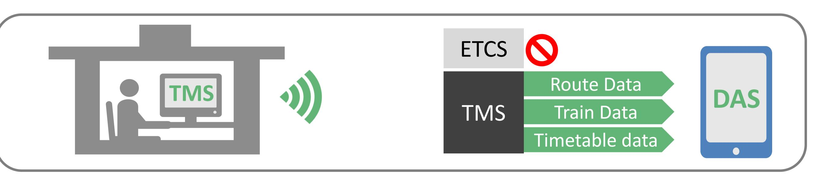
For C-DAS, IM should deliver extra train, infra, timing and communication data
