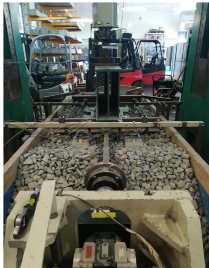
Lateral resistance test configuration Gluing configurations tested
