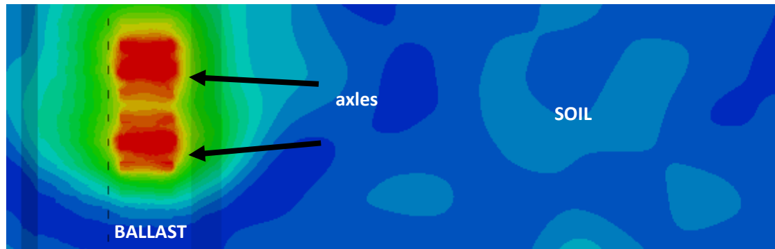
Global displacement magnitude in a pass-by train simulation
